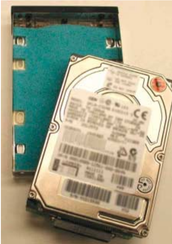
Figure 10: CONFOR CF-EG foam cushion for 2.5-inch hard drive.
