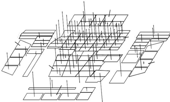
*The arrows on this acoustic map depict the power and direction of sound being introduced by specific sections of the walls, floor and ceiling of the yacht's main lounge/dining area, portrayed here like an unfolded box. These and other measurements are used to customize treatments throughout the yacht.*
