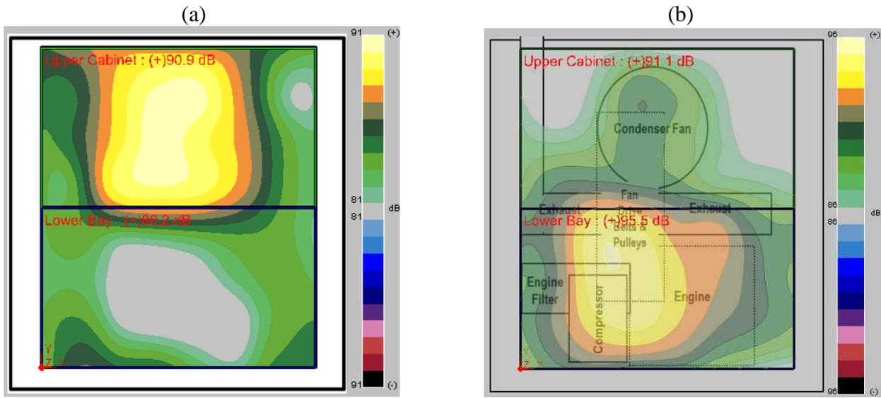
Figure 2: Sound intensity maps with doors closed (a) then removed (b).
