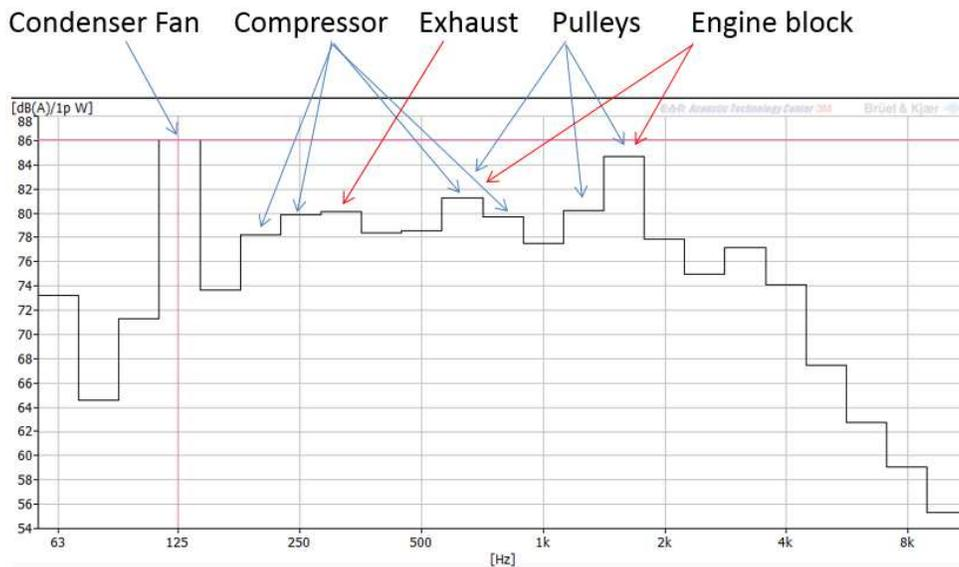
Figure 3: Sound power level spectrum and main noise sources with doors closed.
