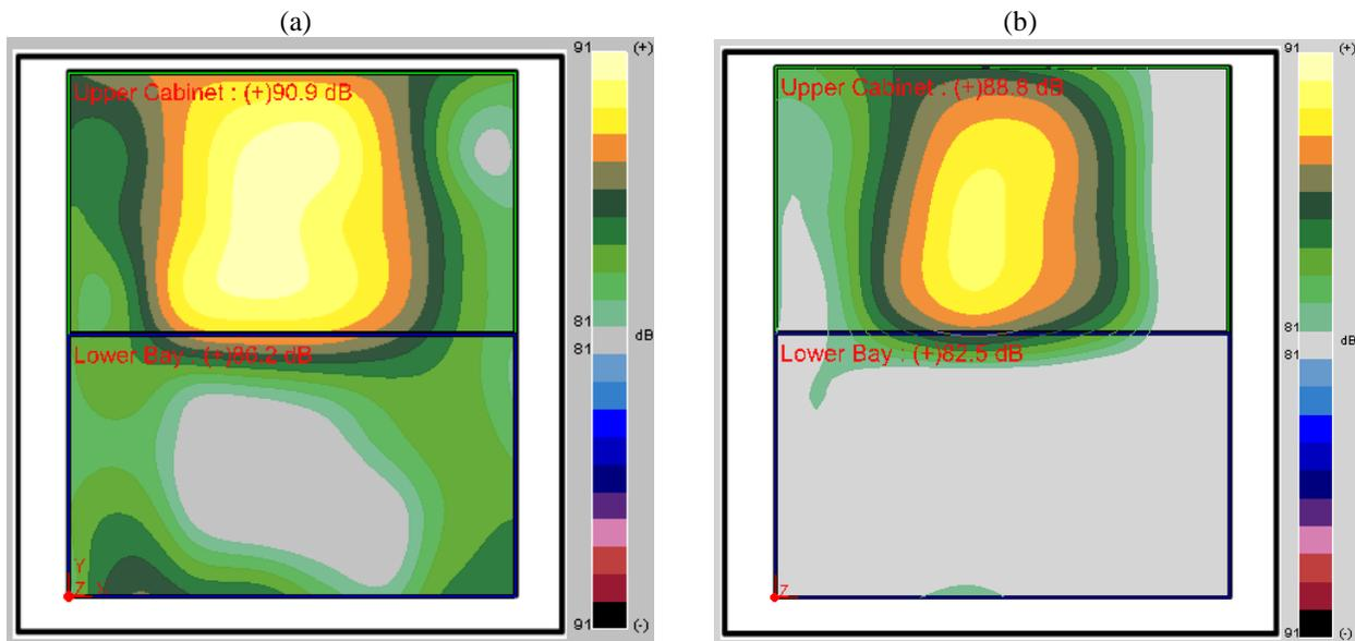
Figure 7: Sound intensity contours of production treatment (a) and optimized package (b).
