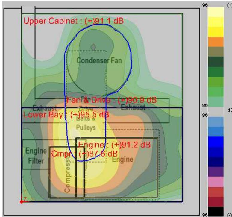
**Figure 4:** Overall sound power levels from each of the main noise sources.
