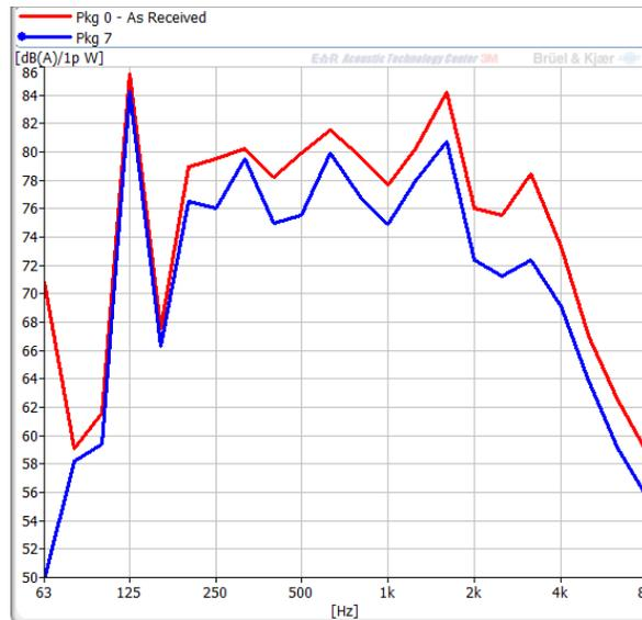
Figure 6: Spectra of production treatment and optimized package (#7).
