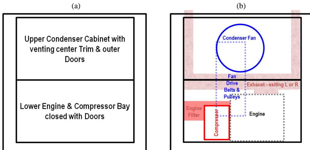
**Figure 1:** Typical layout of exterior (a) and interior (b) components in generic refrigeration unit.
