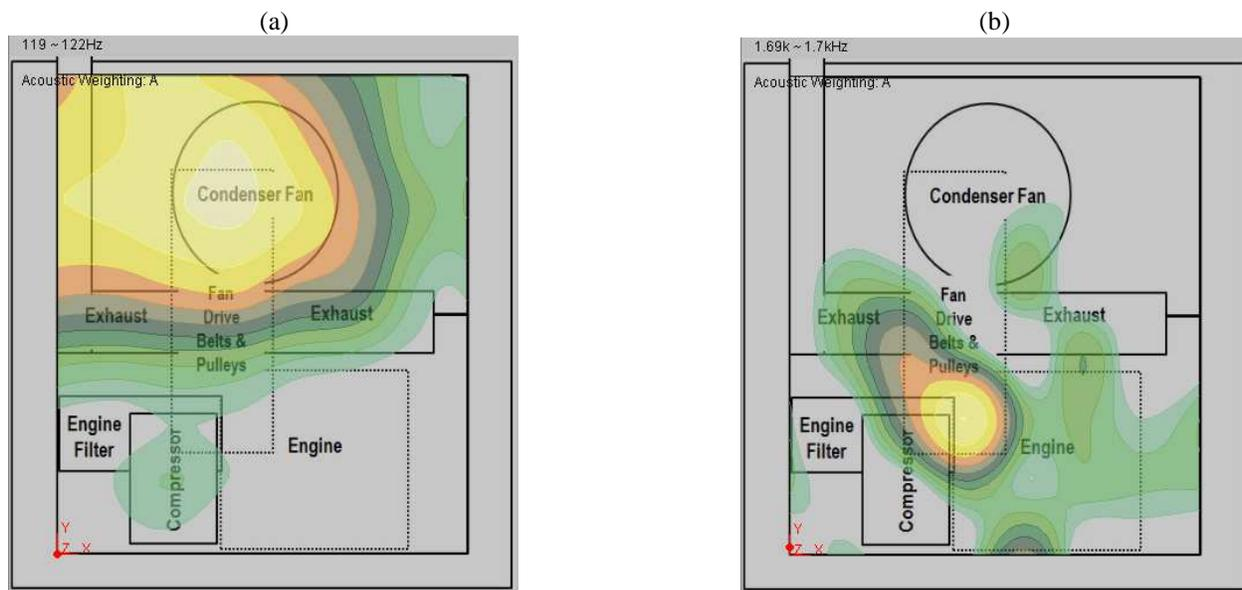
**Figure 5:** Doors removed to show individual sources, at narrow band frequencies, causing high one third octave band levels with doors closed – 125Hz band, condenser fan (a) and 1.6kHz band, lower fan pulley (b).
