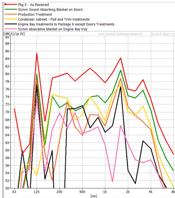
Figure 8: Spectra of radiated sound power as received and power removed by some treatment examples.
