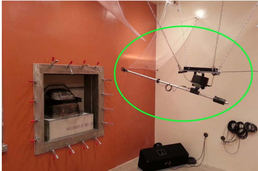
**Figure 3:** Rotating boom diffuse field microphone in receiving reverberation room
