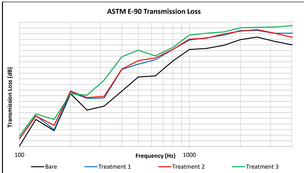
**Figure 6:** ASTM E90 Transmission Loss of Damping Treatments
