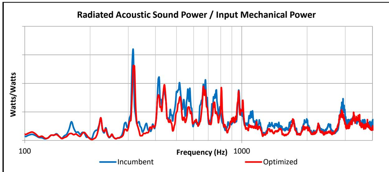
**Figure 4:** Normalized Radiated Acoustic Sound Power of Damping Optimization
