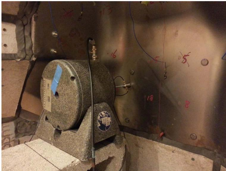
**Figure 2:** Shaker mounted to tunnel via rigid stinger and impedance head
