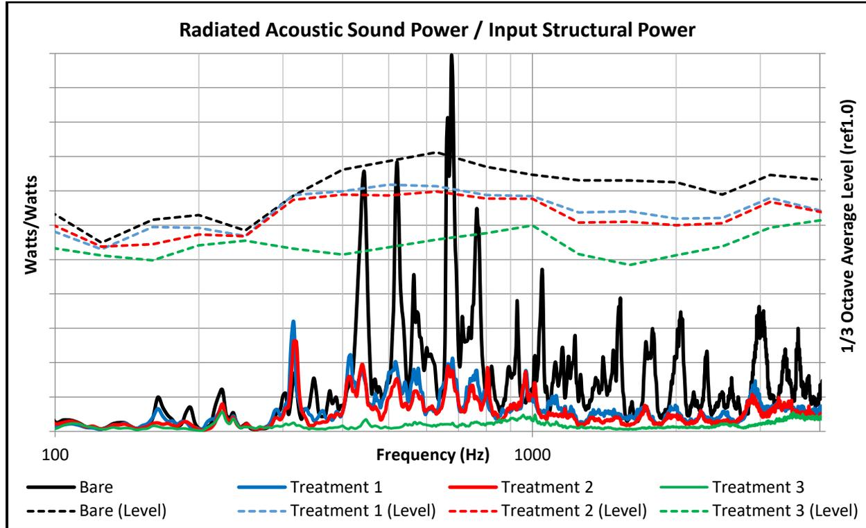
**Figure 5:** Normalized Radiated Acoustic Sound Power of Damping Treatments
