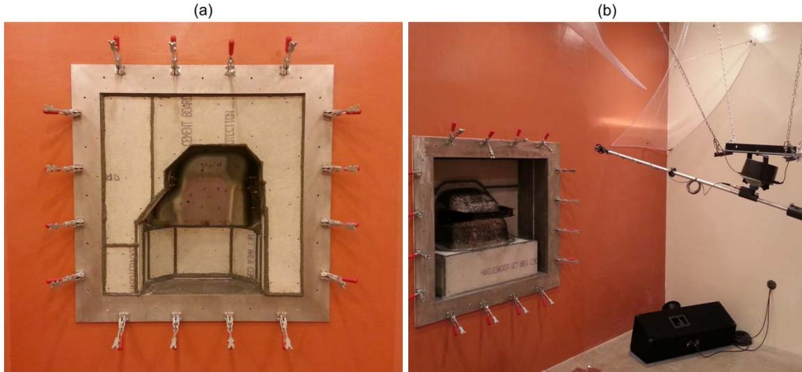
**Figure 1:** (a) Mounted engine tunnel from source room. (b) Mounted engine tunnel from receiving room.
